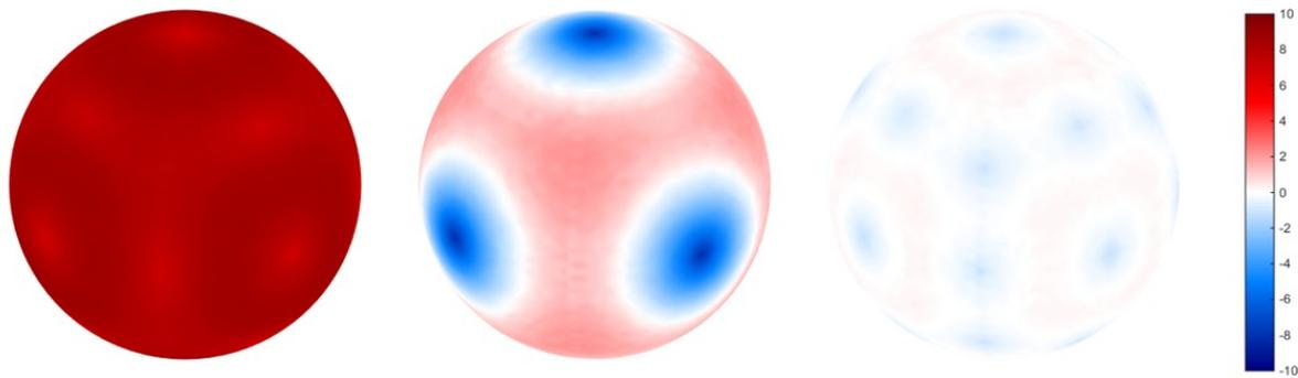
Figure 2. Representation of relative error in surface area measure depending on relative orientation of the shape with image axes (the whiter, the better). From left to right: isosurface, Crofton with three directions, Crofton with 13 directions.
