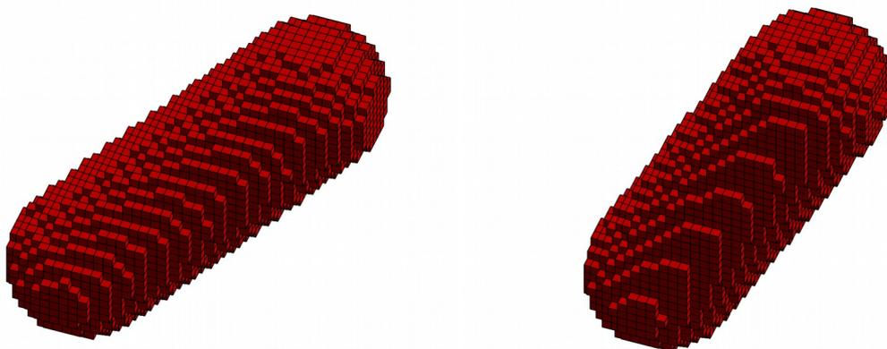
Figure 1. Two different Gauss discretisations of the same 3D binary particle.
