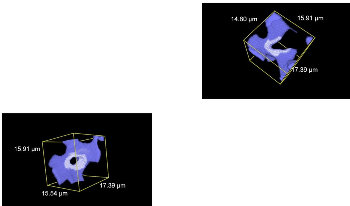
Figure 3. Volume renderings of examples of potential pillars. Using the Euler number, the algorithm correctly detects the right one as pillar and rejects the left one.
