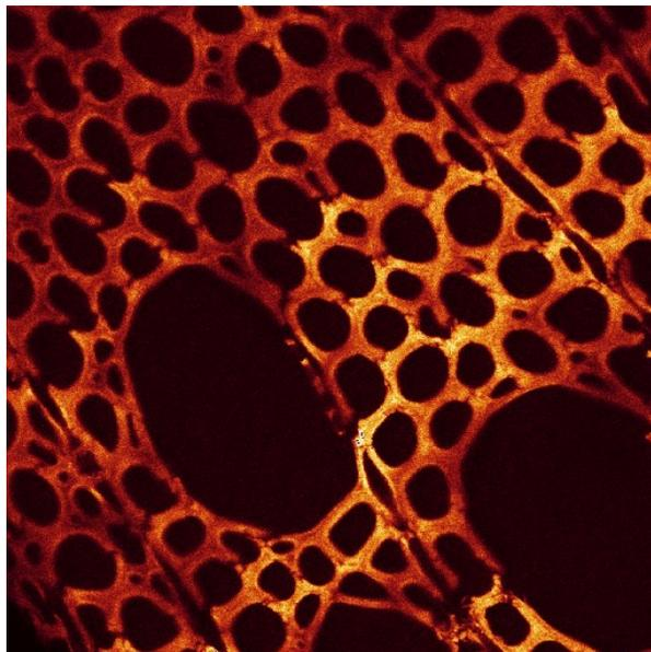
Figure 1. Native poplar section incubated for 24 hours in a 0.2% PEG-RhoB solution observed with a Leica SP2 confocal microscope
