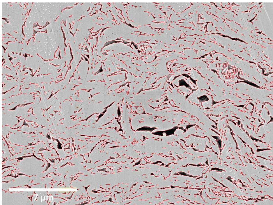
Figure 1. Secondary Electron image showing porosity in clay. Over 5000 pores were segmented (red outline) in this field of view. The measured porosity is 11.95%
