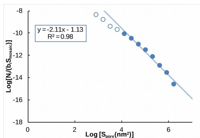
Figure 2. Graph showing power law distribution of porosity measured on SE-Image shown in Figure 1 and normalized by the measured image area. Segmentation is assumed to be valid for pores larger than 9 pixels which corresponds to  $\sim 10^4 \text{ nm}^2$  at the given image resolution.
