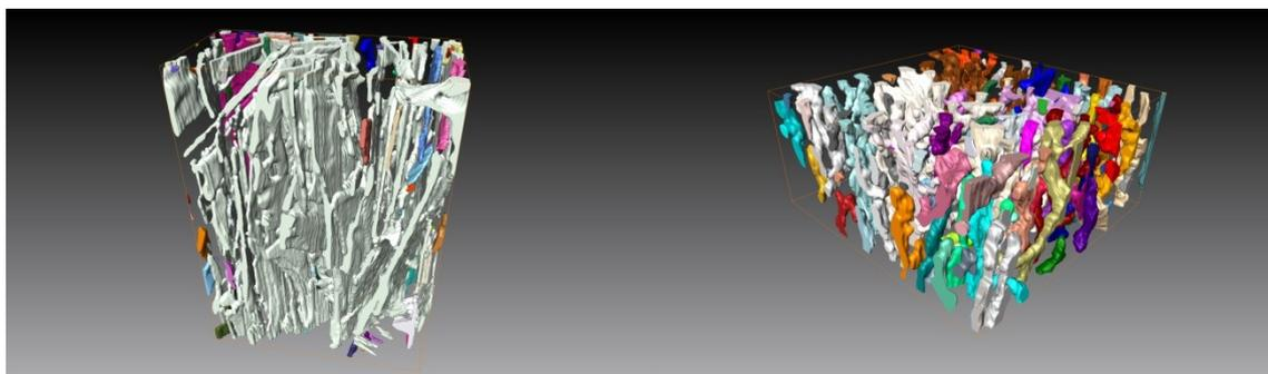
Figure 1. Reconstructions from FIB/SEM tomography. (Left) Interconnected, plate like silicon in the unmodified Al-7wt%Si alloy and (right) coral like morphology of the eutectic silicon in the Sr-modified alloy.
