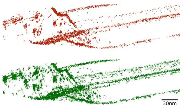
Figure 2. Reconstruction from atom probe tomography. Aluminium (green) and Strontium (red) rich structures in eutectic silicon of the Sr-modified Al-7wt%Si alloy.
