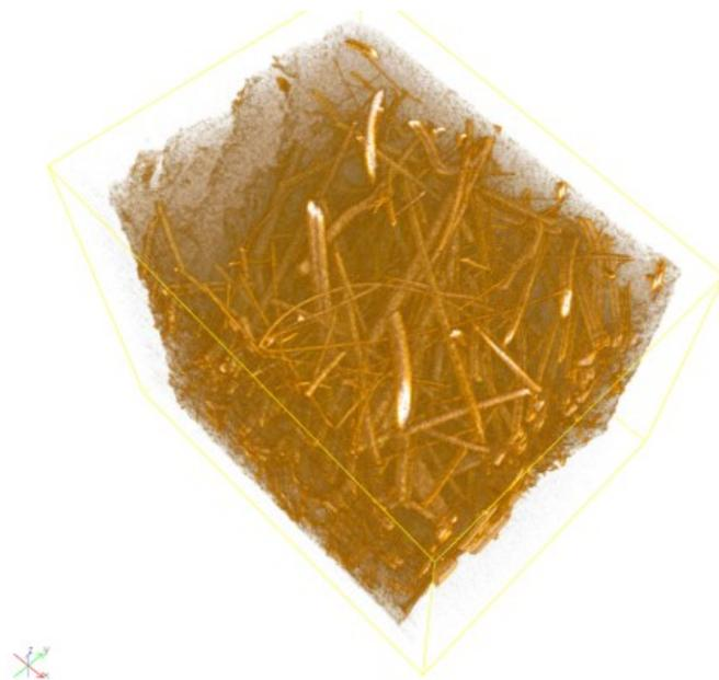
Figure 1: Visualization of CT image (550 nm pixel spacing and approximately 0.5 mm side length) (Data provided by MANN+HUMMEL GMBH, Ludwigsburg , CT imaging by RJI Micro & Analytic GmbH)
