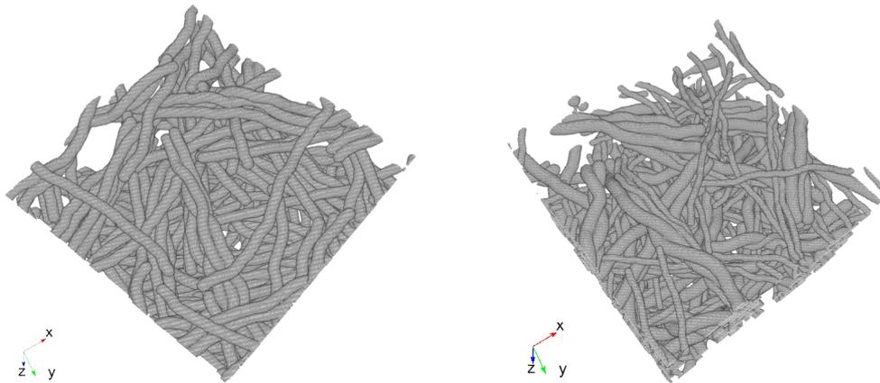
Figure 2: Realizations of the new fiber system model with fiber diameter 10 pixels and with fiber diameter 6 and 12 pixels
