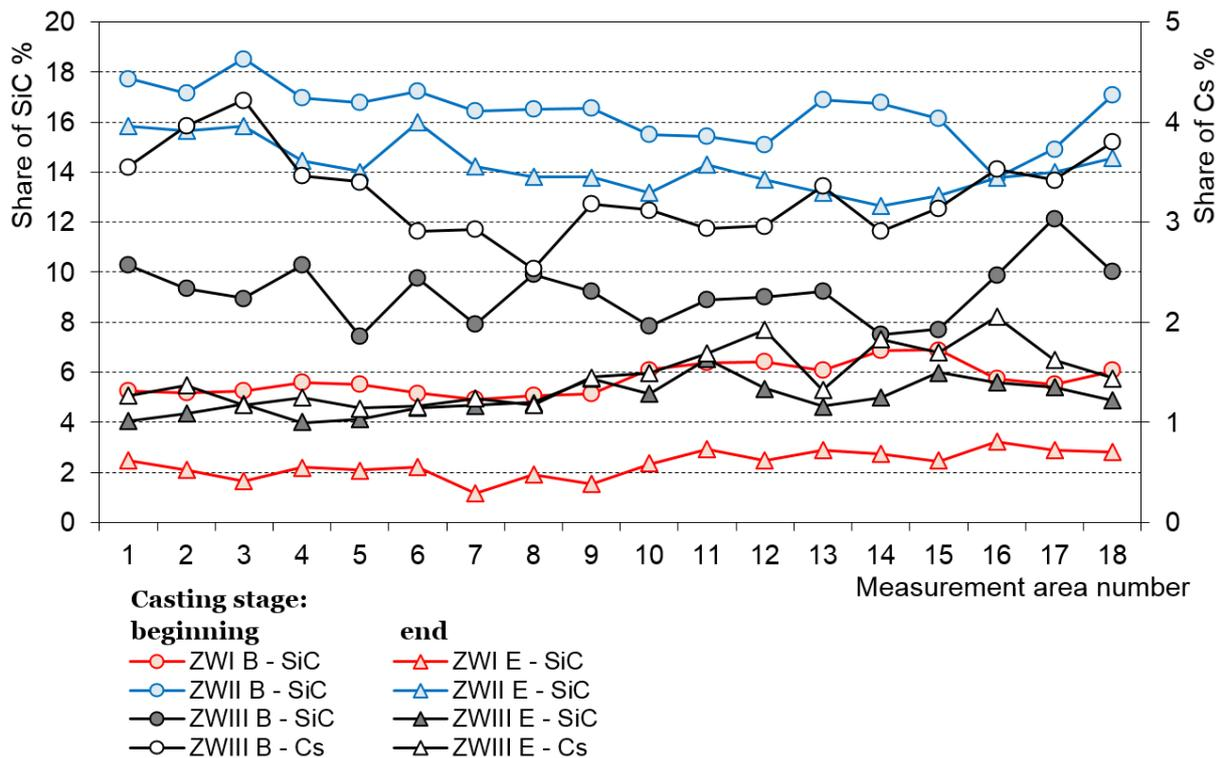
Figure 5. Percent content of the reinforcing particles of SiC and Cs in the examined ZWI, ZWII and ZWIII pistons
