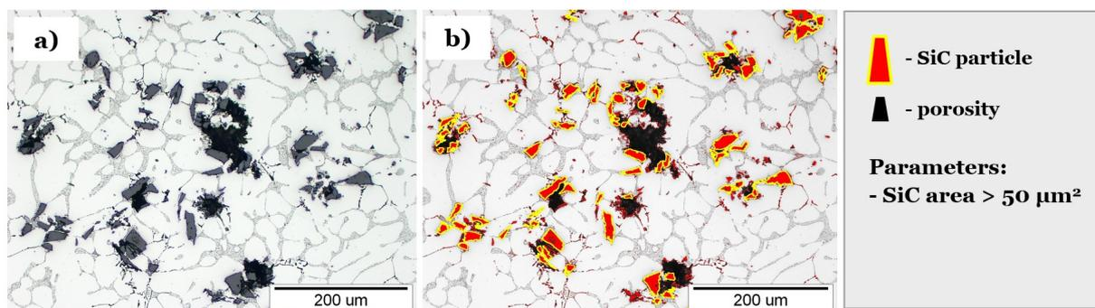
Figure 3. Example of microstructure obtained in ZWI piston (a) with marked SiC particles (b)
