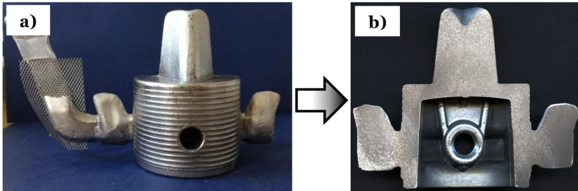
Figure 1. Cast piston (a) and its cross-section (b)
