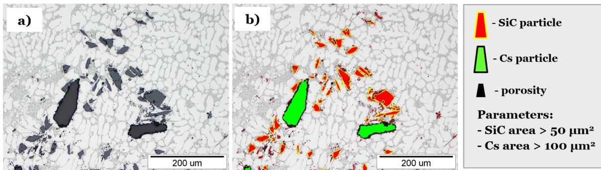
Figure 4. Example of microstructure obtained in ZWIII piston (a) with marked particles of SiC and Cs (b)
