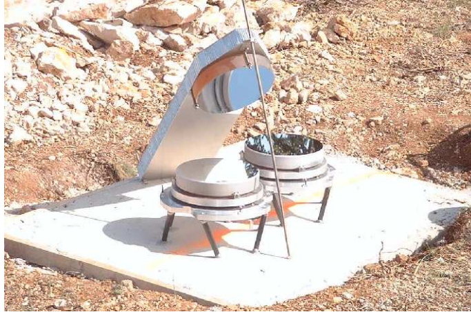
Figure 1: Initial testing configuration with two 25cm mirrors arranged in close spacing and a folding flat mirror for metrology at the curvature center. The two spherical mirrors are partially covered by the flat mirror making the curvature center easily accessible at ground level, 70 meters away. The mirror supports are rigidly anchored to the bed-rock via concrete and carbon fiber tubes.
