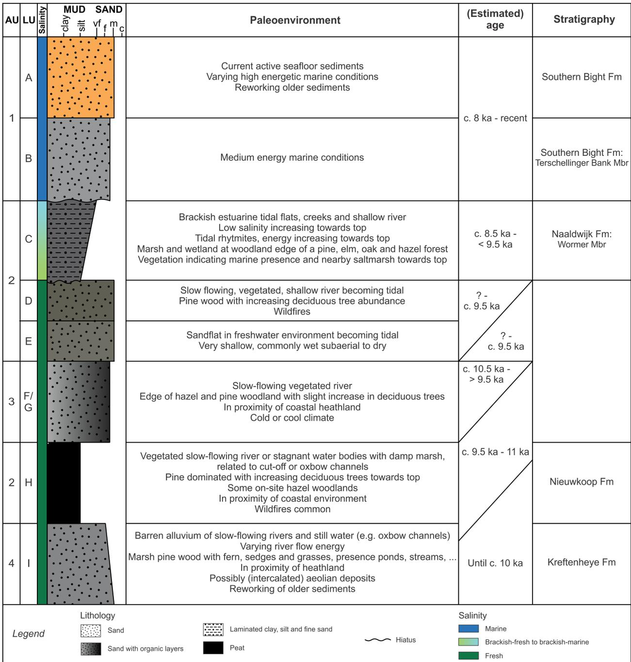
**Figure 2.** Conceptual model of the paleoenvironmental evolution of the Brown Bank area based on a composite log of all encountered lithological units (LU) and their corresponding acoustic units (AU). Fm = Formation; Mbr = Member.
