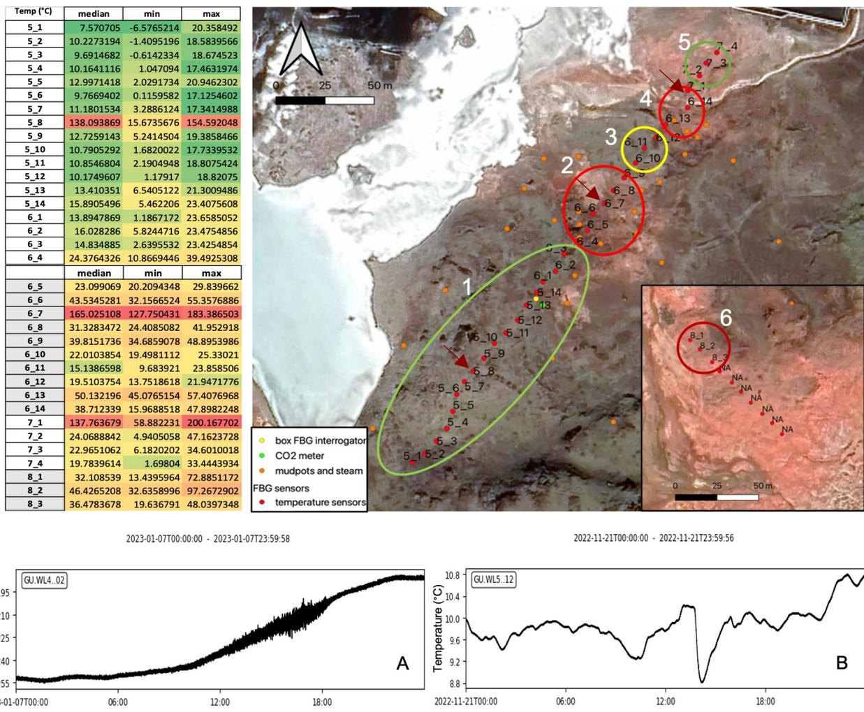
**Figure 1.** Top: Soil temperature distribution map. Six different temperature zones (ellipses) were identified in the field. Red arrows indicate sensors with anomalously high temperature readings. Table shows median, minimum and maximum temperature values recorded by the temperature sensors throughout the study period (in °C). Temperatures are color-coded: green = lowest temperature, red = highest temperature. Bottom: A) Thickening in strain signal; B) Jump in temperature signal.
