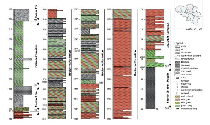
Figure 3. Litholog of the Devonian of borehole 059E146 (KB132, Booischot), stratotype of the Booischot Formation. Lithology based on detailed litholog from Legrand (1964), Bless et al. (1976), Langenaeker (2000) and Coen-Aubert (2014). GeoDoc 059E146.
