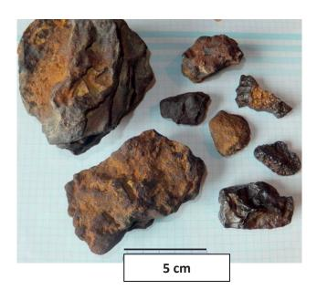
Figure 14. Picture of the iron concretions found in the concentrated layer at Beerzel. The concretions to the right clearly have a polished surface.
