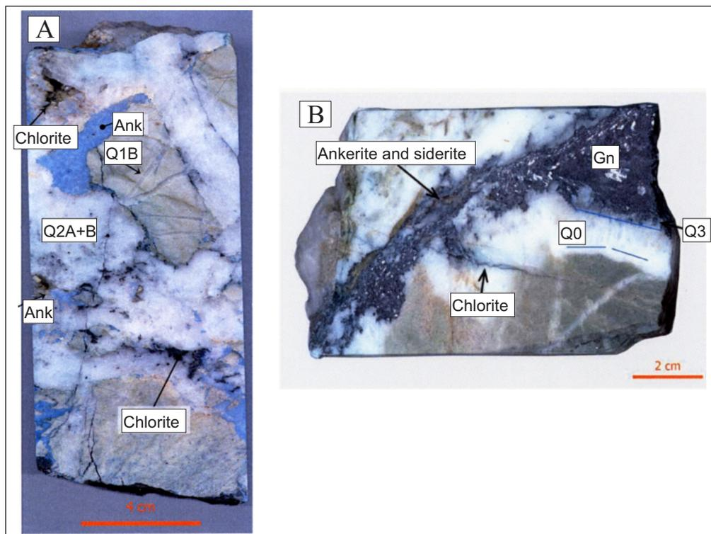
**Figure 3.** A. Sample from 1593 m depth of borehole 171W276 at Grand-Halleux, indicating different quartz and carbonate generations. B. Sample from 2253 m depth of borehole 171W276 at Grand-Halleux, indicating relationship between galena mineralization (Gn) and different quartz (Q0, Q1B, Q2A+B, Q3) and carbonate vein generations (Ank: ankerite).
