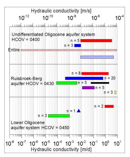
Figure 10. Horizontal hydraulic conductivity ranges for the Oligocene aquifer system (HCOV 0400) using different measurement methods, showing the number of measurements per method (n), including the proposed range for use in groundwater modelling. Ranges from other sources include values documented in Brulandkrijt System (VMM, 2008b) and SAFIR 2 (ONDRAF/NIRAS, 2001). Same legend as in Fig. 6.
