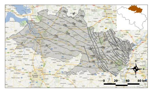
Figure 1. Extent and depth of the base (in m TAW; Tweede Algemene Waterpassing) of the Boom Formation in Belgium (based on interpretations of the Geological Survey of Belgium (Vancampenhout, 2004: Welkenhuysen et al., 2012)). Faults cross-cutting the Boom Formation are shown by NW-SE trending lines; they belong to the Roer Valley Graben system. A map of Belgium with the location of the Boom Formation is shown in the upper right corner.
