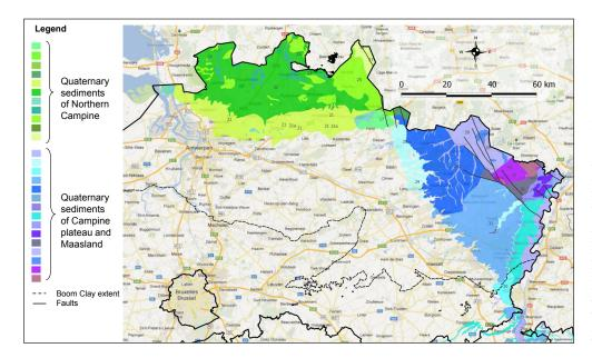
Figure 2. Hydrogeologically significant Quaternary sediments. The sediment profile types of the Northern Campine (greenish colours) correspond roughly to the Campine complex (HCOV 0220), the sediment profile types of the Campine plateau and the (bluish Maasland colours) correspond to the Maas and Rhine deposits (HCOV 0170) and to the sediments north of the Feldbiss fault (HCOV 0210). Based on the Quaternary geological map of Databank Ondergrond Vlaanderen.
