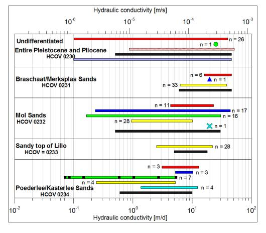
Figure 7. Horizontal hydraulic conductivity measurement ranges for the Pleistocene and Pliocene aquifer (HCOV 0230), together with the number of measurements (n), including the proposed ranges for use in groundwater modelling. Ranges from other sources include the Central Campine System (VMM, 2008a) and SAFIR 2 (ONDRAF/NIRAS, 2001). Same legend as in Fig. 6.
