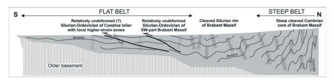
Figure 4: Schematic section from the (thick) central part of the Brabant Massif towards the (thin) Condroz Inlier, demonstrating the transition from a steep belt towards a flat belt, typical for many orogens (not to scale).
