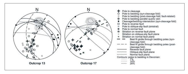
**Figure 3:** Lower-hemisphere equal area projections of bedding, cleavage, cleavage/bedding intersection and fault data of outcrops 13 (cf. fig. 2A & 2B) and 17 (cf. fig. 2C & 2D) of Vanmeirhaeghe (2006). For comparison, contours of poles to bedding in the Devonian of the Dinant Synclinorium are added (grey-shaded contours in background; outcrops 1 & 2 of Vanmeirhaeghe, 2006).
