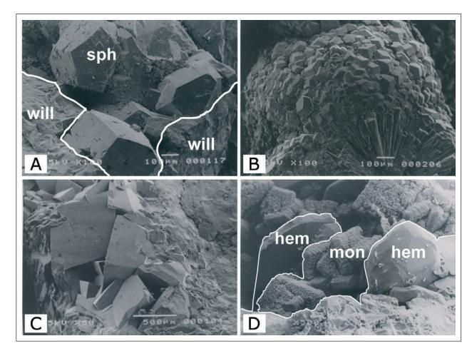
**Figure 2:** SEM micrographs of willemite and smithsonite samples. A. La Calamine: willemite (will) replaces sphalerite (sph) crystals; B. La Calamine: microcrystalline terminations of willemite spheroids in botryoidal aggregates; C. La Calamine: smithsonite idiomorphs filling a vein in willemite; D. Fossey: Fe-smithsonite (monheimite) among hemimorphite laths. Collections of the Royal Belgian Institute of Natural Sciences, Brussels.
