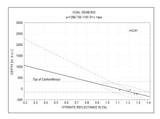
Figure 5. Relationship between vitrinite reflectance and depth in coal seam 833. Thickness of eroded Carboniferous beds, equal to about 800 m, was determined under the assumption that the top of the Carboniferous strata occurs at a depth of 250 m ( $\sim$ 1050 m - 250 m =  $\sim$ 800 m).
