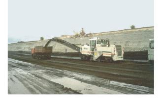
Figure 10. Wirtgen Machine stripping lignite in Pit B, Gacko mine.
