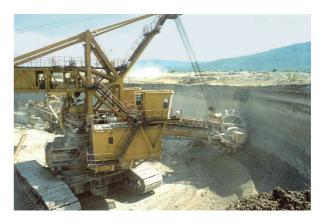
Figure 9. Bucketwheel Excavator cutting overburden at Gacko Mine.
