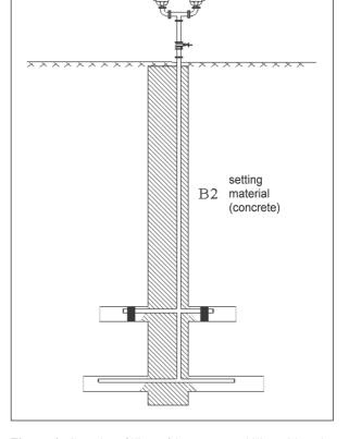
**Figure 4**: Complete filling of long-term stability with a degasification pipe.
