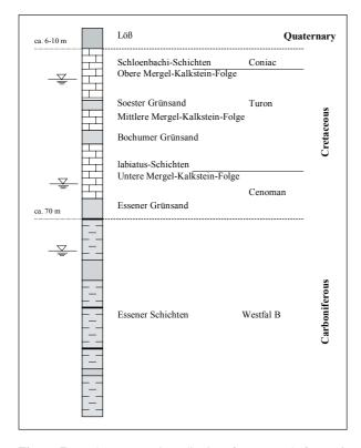
**Figure 7**: Rock sequence in a district of Dortmund (figure 6, borehole D).
