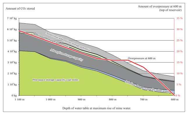
**Figure 9.** The sequestration capacity of the Anderlues colliery for different amounts of overpressure, assuming that the shafts are sealed at a depth of about 600 m. Calculation with  $CO_2$ -VR (Piessens & Dusar, 2003c). X-axis: depth of the water table; leftmost Y-axis: amount of sequestered  $CO_2$ ; right Y-axis: amount of overpressure at the top of the reservoir (600 m), in percentage relative to the hydrostatic pressure.
