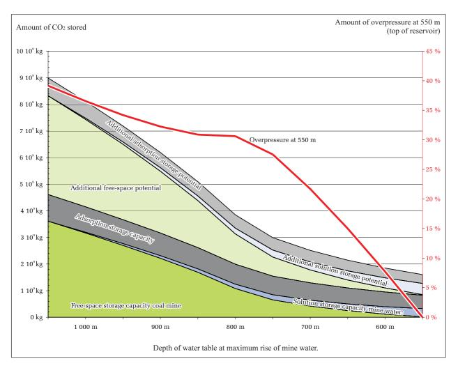
**Figure 7.** The sequestration capacity of the Beringen colliery for different amounts of overpressure on the top seal. Calculation with  $CO_2$ -VR (Piessens & Dusar, 2003c). X-axis: depth of the water table; leftmost Y-axis: amount of sequestered  $CO_2$ ; right Y-axis: amount of overpressure at the top of the reservoir (550 m), in percentage relative to the hydrostatic pressure.
