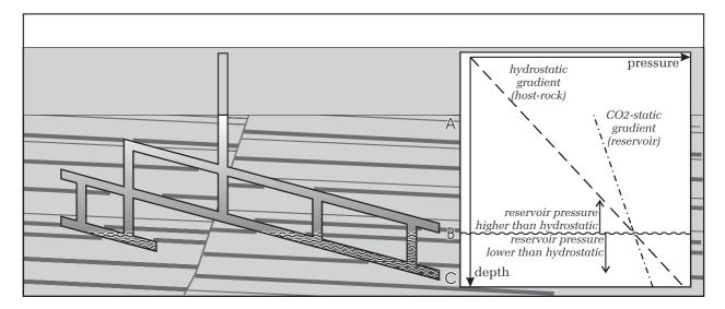
**Figure 3.** Schematic representation of a mine reservoir and the pressure evolution in the mine reservoir and the hosting formations. The reservoir is in overpressure relative to the hydrostatic gradient between points A and B, and in equilibrium with the hydrostatic pressure between B and C.
