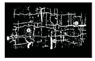
**Figure 8.** Detected in white, open cleats (C), mineral filled fractures (M) and bedding (B).
