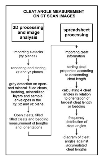
**Figure 6.** Flow chart of the image analysis procedure to define fracture angles from CT scans.
