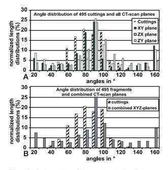
**Figure 9 A,B.** Comparison of cleat angle results from fragments and CT scans. A: Fragments versus the CT-scan XY- plane and reconstructed ZX- and ZY- planes. B: Fragments versus the combined CT-scan XY, ZX and ZY planes.
