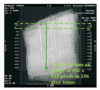
Figure 4. X-ray view on the top of sample 495. The arrow shows the scans according to the Z- direction.
