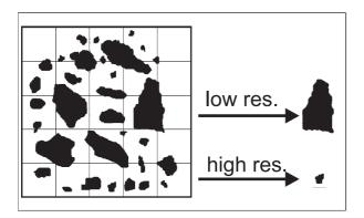
Figure 2. From a fragment aggregate to single fragment images at different resolutions.
