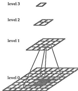
Fig.1. A  $2^3 \times 2^3$  overlapped pyramid.
