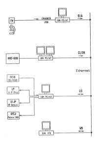
Fig. 2. Block scheme of the open, semi-automatic sterelogical image analyzer and I/O image devices connected Ethernet (CFEJ: colour film exposition control unit; CIJP: colour ink-jet printer; CLSM: confocal laser scanning micro-GS: scope; graphic station; FCIS: flat-bed colour image LP: scanner; laser printer; SIA: semi-automatic image analvzer; WS: Unix workstation.
