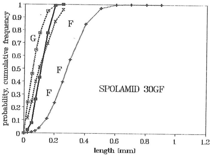
Fig.3. Probability distribution of length F, experimental pull-out length  $F_e$ , theoretical pull-out length G (model A) and computer simulated distribution  $F_s$  (model B).
