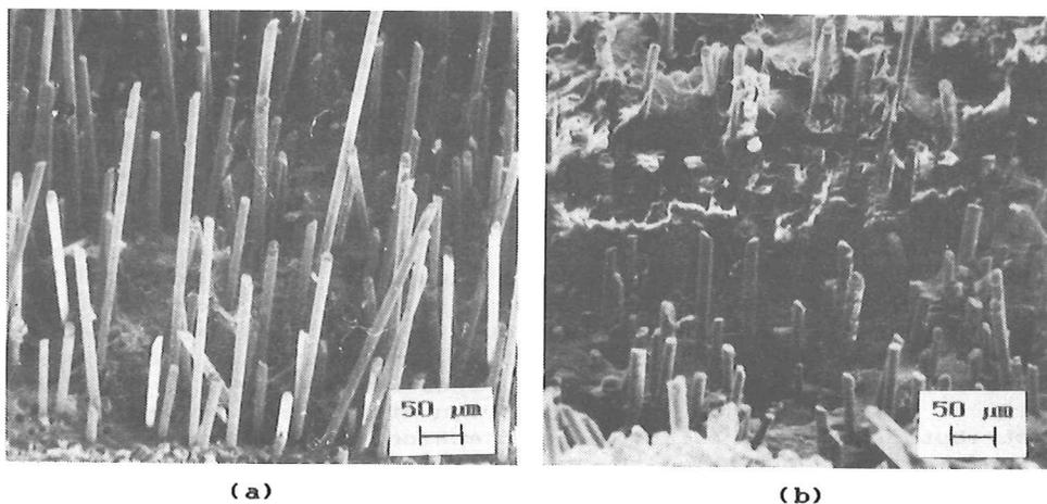
Fig.1. Scanning electron micrographs of fractured specimens of injection moulded glass fibre reinforced plastics:
