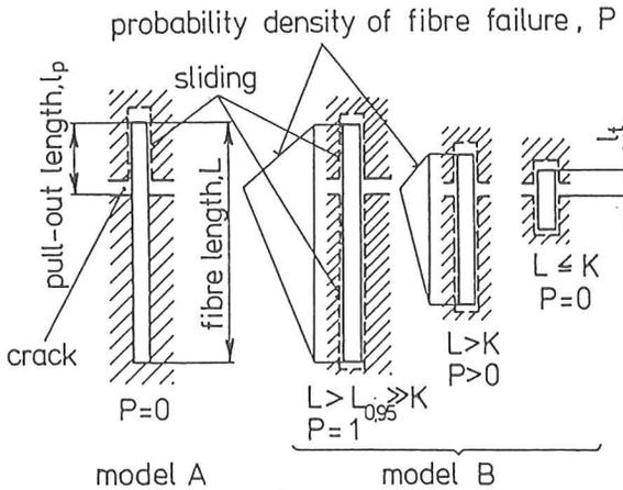
Fig.2. Schematical diagram of short fibre composite fracture ahead of a notch. Model A - without fibre failure and one-side sliding of fibre, model B - with fibre failure and two-side sliding.
