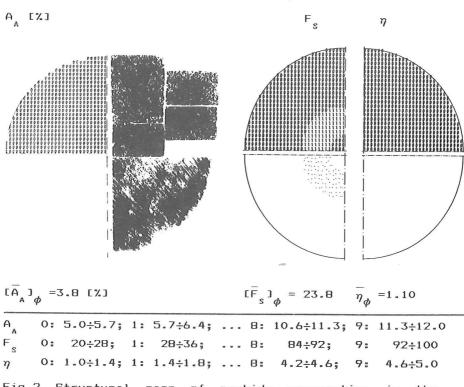
Fig.2. Structural maps of carbide segregation in the SC 0-5-1-2Ti steel bar of diameter of 130 mm.
