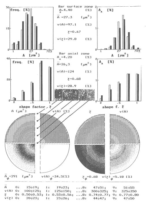
Fig.4. Quantitative characteristic of carbide particles size and shape in SC 0-5-1-2Ii steel  $\phi$  130 mm bar (forging reduction ratio = 2.9)
