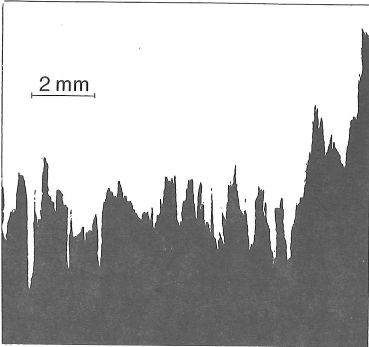
Fig.4. Fracture profile of the broken pine board.
