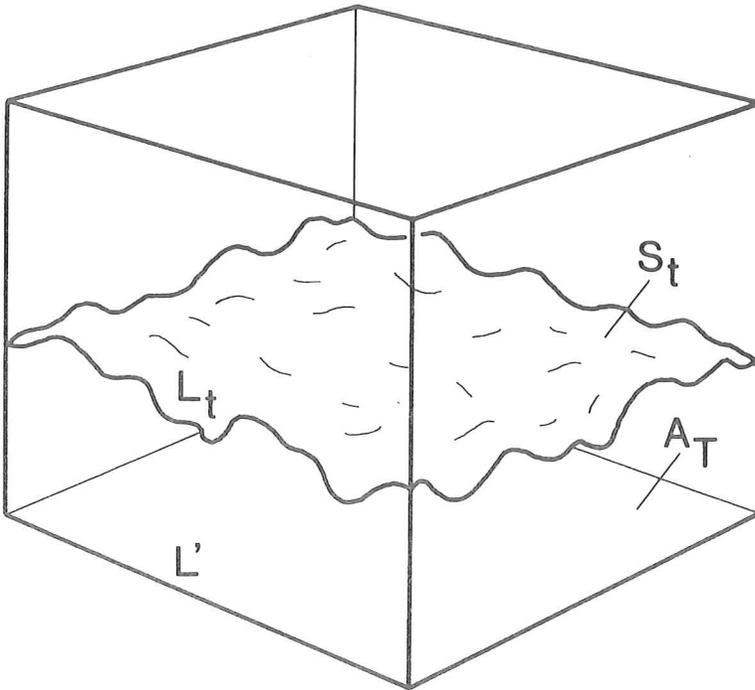
Fig.1. Test cube, fracture surface and fracture profile.
