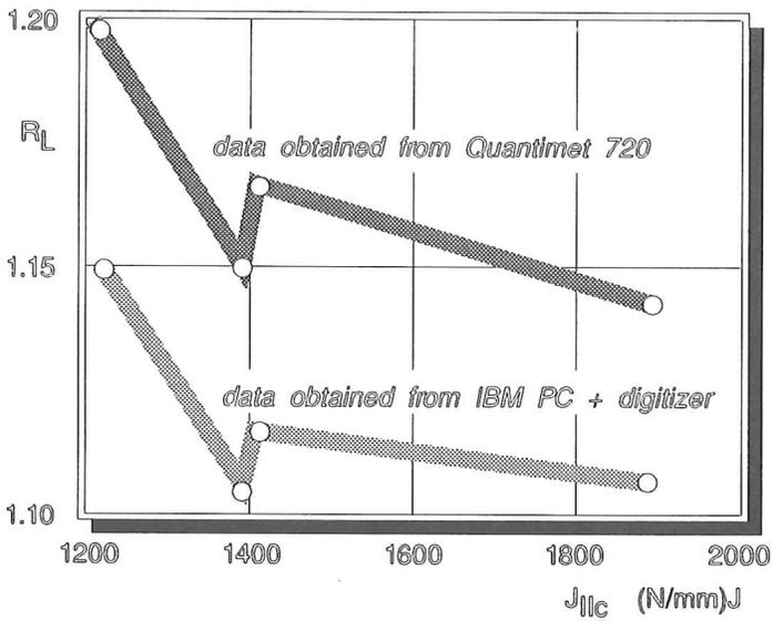
Fig.1. Profile line parameters versus work of fracture
