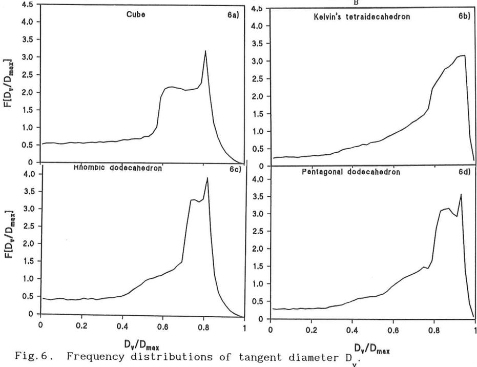
Fig.6. Frequency distributions of tangent diameter  $D_v/D_{max}$ .
