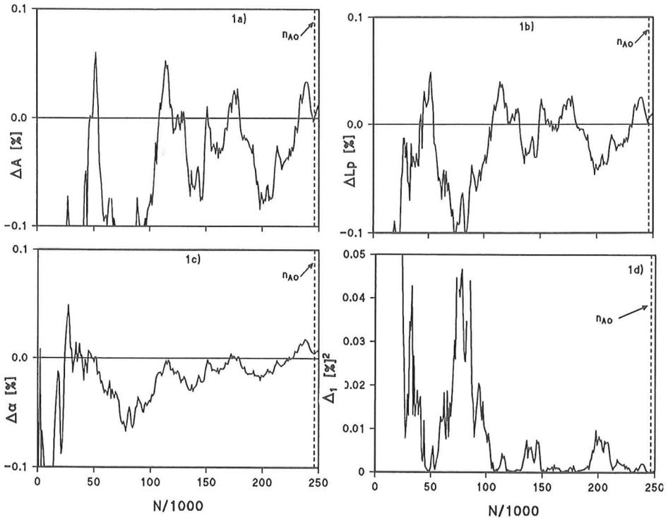
Fig.1. Dependence of errors of area of section  $\Delta A$ , plane angle  $\Delta\alpha$ , perimeter  $\Delta L_p$  and  $\Delta_1$  as a function of the number of sections of Kelvin's tetraidecahedron. Note:  $n_{AO} = 246,187$ .
