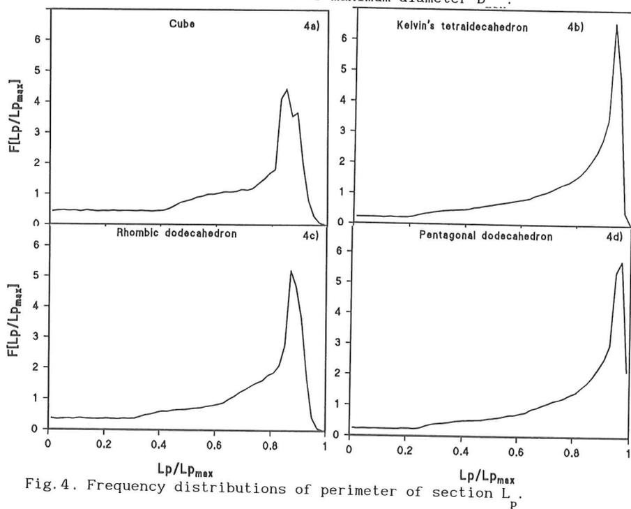
Fig. 4. Frequency distributions of perimeter of section  $L_p$ .
