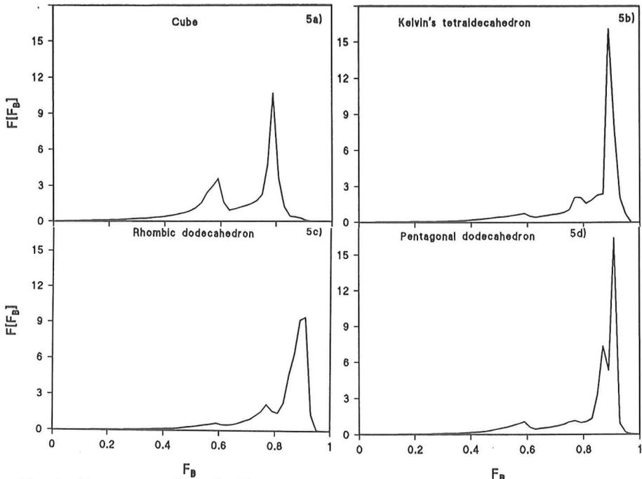
Fig.5. Frequency distributions of shape coefficient  $F_B$ .
