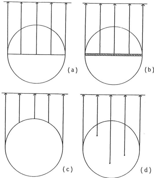
Fig. 1. Possibilities for obtaining an image of an object in the (a) optical or (b) physical sectioning, (c) projection from the surface, (d) projection from the interior (after Kališnik and Obrez, 1987).
