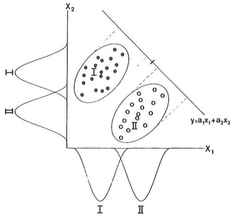
Fig. 3. Bivariate analysis of two samples I and II (which produce overlapping in separate analysis of variables  $X_1$  and  $X_2$ ), enabling complete separation of both samples (with permission after Baak and Oort, 1983).
