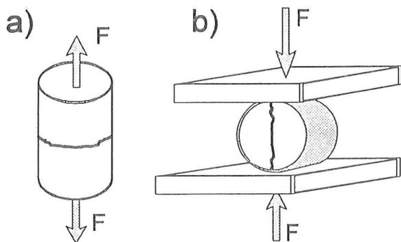
Fig. 1. A scheme of a tensile test of the samples: (a) direct tension, (b) indirect - brazilian test
