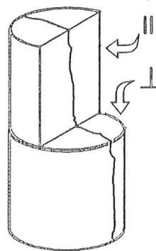
Fig. 2. Location of the cutting planes.
