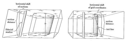
Fig. 3. If improper realignment because of horizontal shifts (left picture) is reversed to restore the original position (right picture), then the length of test lines between two sections increases.
