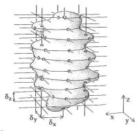
Fig. 2. The apparent surface area is estimated using a spatial grid with spacings  $\delta_X$ ,  $\delta_Y$  and  $\delta_Z$ .
