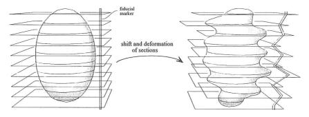
Fig. 1. Improper realignment and deformation of sections lead to seeming surface area increase.
