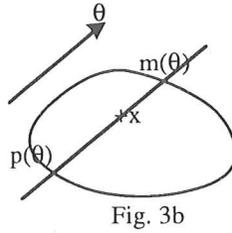
Support lines of direction  $\theta$  and a chord of direction  $\theta$  through  $x$
