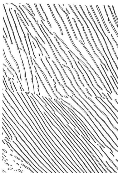
Fig.6. Microstructure of the pearlite in model alloy used in experiments.
