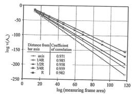
Fig. 1. Log-log plot of coefficient of variation of carbide particles area fraction, measuring frame area in systematic scaning and variance analysis method.
