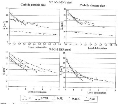
Fig. 6. Effect of local deformation on carbide particles and clusters size.
