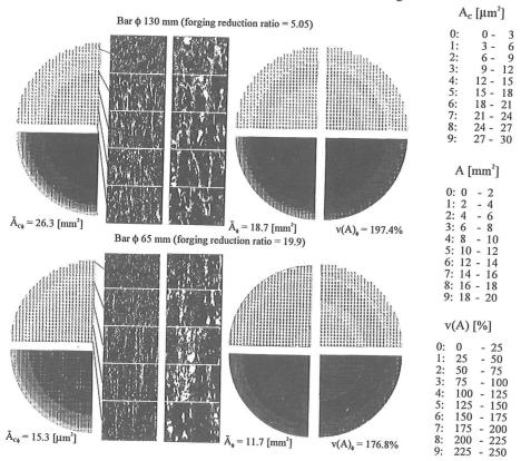
Fig. 2. "Structural maps" showing the effect of forging reduction ratio on carbide clusters and particles size variation on transverse cross-section of SC 1-5-1-2Nb high-speed steel bars.
