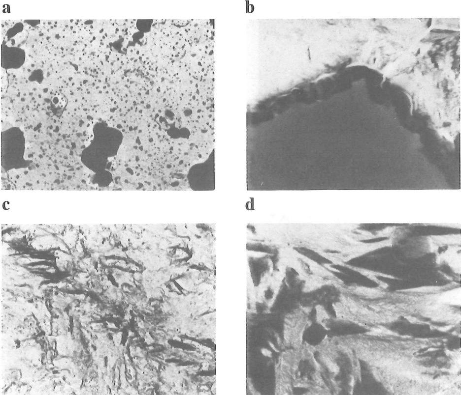
Fig.4. Carbide particles in nonledeburitic HSS (TEM):
