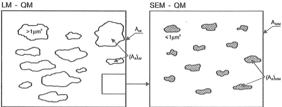
Fig.1. Scheme of A<sub>A</sub> assessment by LM + SEM - QM method.
