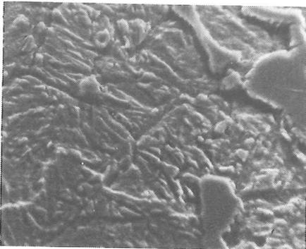
It is visible that possibility of automatic detection and consecutive measurements of carbide particles while using LM are restricted solely to large ( $> 1 \mu\text{m}^2$ ) primary MC type carbides. Therefore, SEM images were employed to assess properly smaller ( $\leq 1 \mu\text{m}^2$ )  $\text{M}_6\text{C}$  type carbides in as-annealed and as-hardened steel (undissolved ones) as well as fine dispersion of  $\text{M}_{23}\text{C}_6$  type secondary carbides in as-tempered steel (Fig.3).
