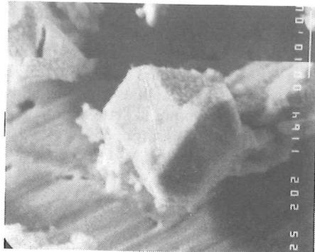
Fig.3. Carbide particles in nonledeburitic HSS (SEM, SEI):
