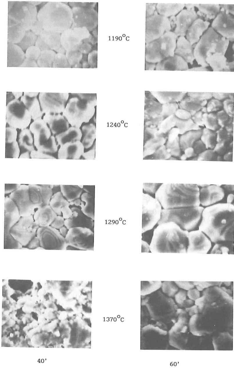
Fig.2 SEM microstructures of BaTiO<sub>3</sub> - ceramic samples (x5000).
