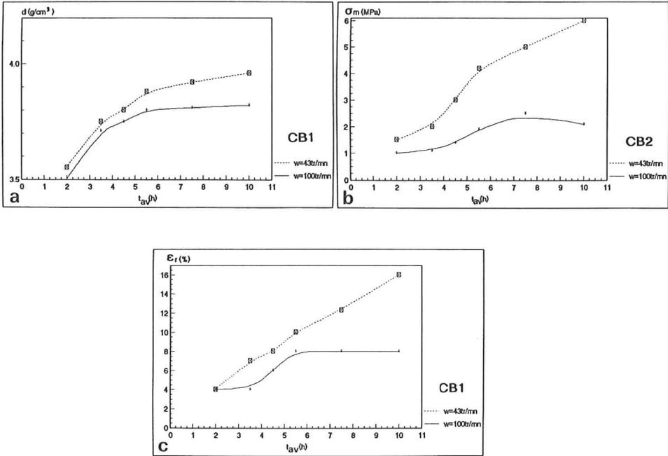
Figure 3 :Change in some characteristics of the green material with the milling conditions (rotating speed of the jar,  $w$ ) as a function of the milling time,  $t_{av}$  : a) density,  $d$  ; b) maximum tensile stress,  $\sigma_m$ ; c) strain to rupture,  $\epsilon_r$ . The curves correspond, for each figure, to texture  $T_1$  and  $T_4$  (respectively  $w = 43$  tr/mn and  $100$  tr/mn).
