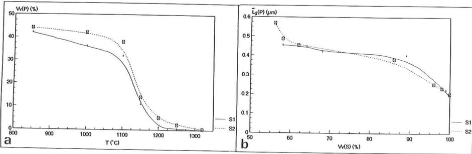
Figure 4 : Change in the volumic fraction of pores,  $V_v(P)$ , as a function of the sintering temperature,  $T$ , and of the mean length of pores,  $L_1(P)$ , as a function of the volumic fraction of solid,  $V_v(S)$ , for two types of texture,  $T_1$  and  $T_4$  (noted  $S_1$  and  $S_2$  respectively), of initially different homogeneity.
