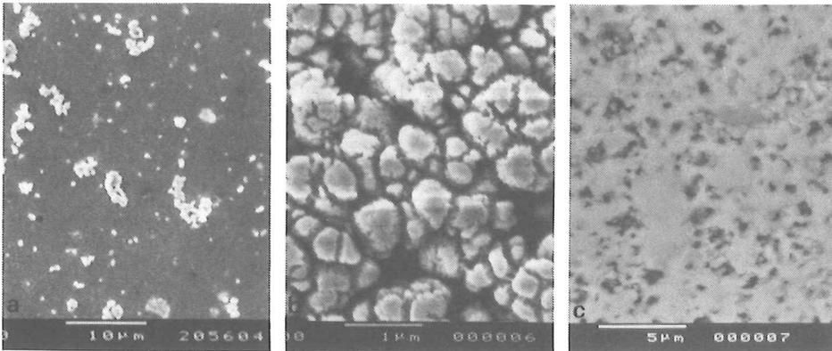
Figure 1 : Micrographs of : a) BaTiO<sub>3</sub> powder ; b) green film, texture T4 ; c) sintered parts, S<sub>1</sub>, at 1150°C.
