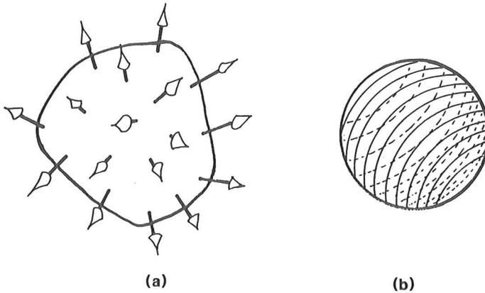
Figure 2. The set of normals for a smooth, closed convex surface (a) map as a set of spherical images that cover the unit sphere of orientation exactly once (b).
