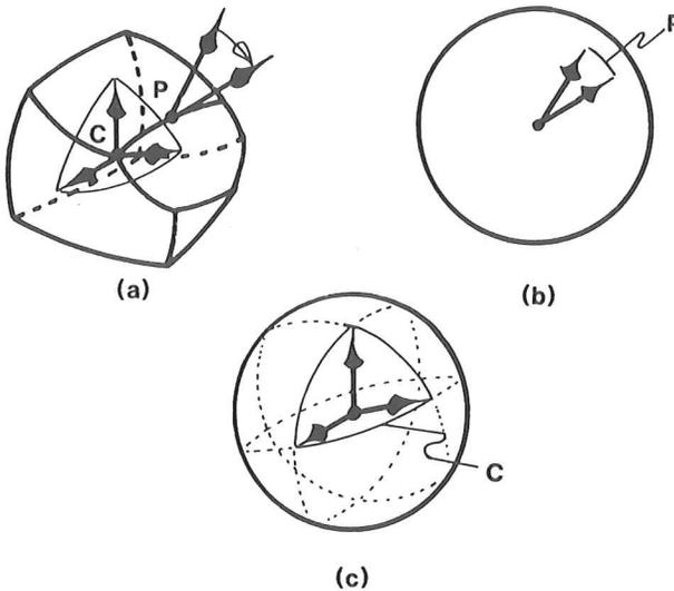
Figure 3. The spherical image of a point P on an edge of a polyhedron (a) maps as a segment of a great circle (b). The spherical image of a corner of a polyhedron (a) is a spherical polygon (c).
