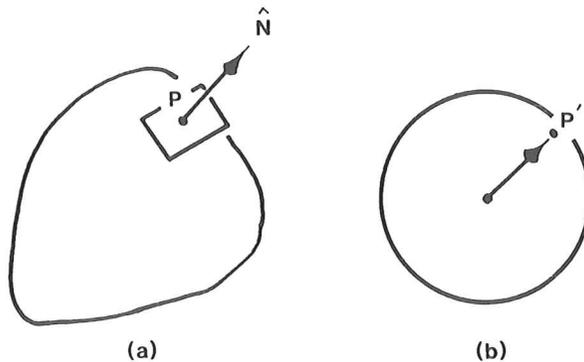
Figure 1. A point  $P$  on a smooth surface has a unique tangent plane and surface normal (a);  $P'$  is the spherical image of  $P$  (b).
