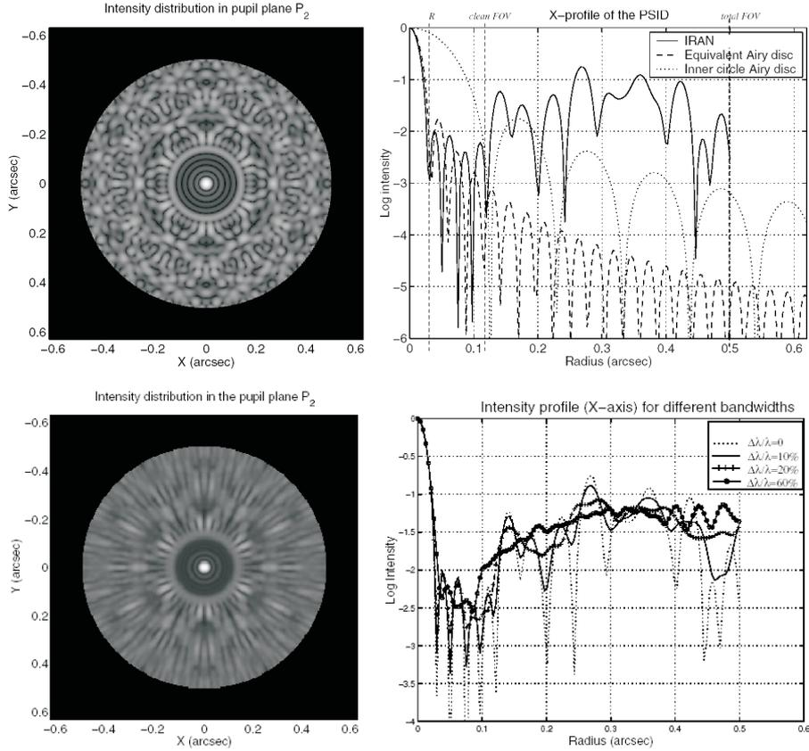
Figure 3: The focal diffraction pattern of KEOPS from 39 co-phased telescopes. Using image-densification (Vakili, et.al 2004), it is possible to reconstruct a pseudo-Airy pattern in the pupil plane, with true convolution relation with the object. On top: monochromatic PSF, bottom: effect of bandwidth.
