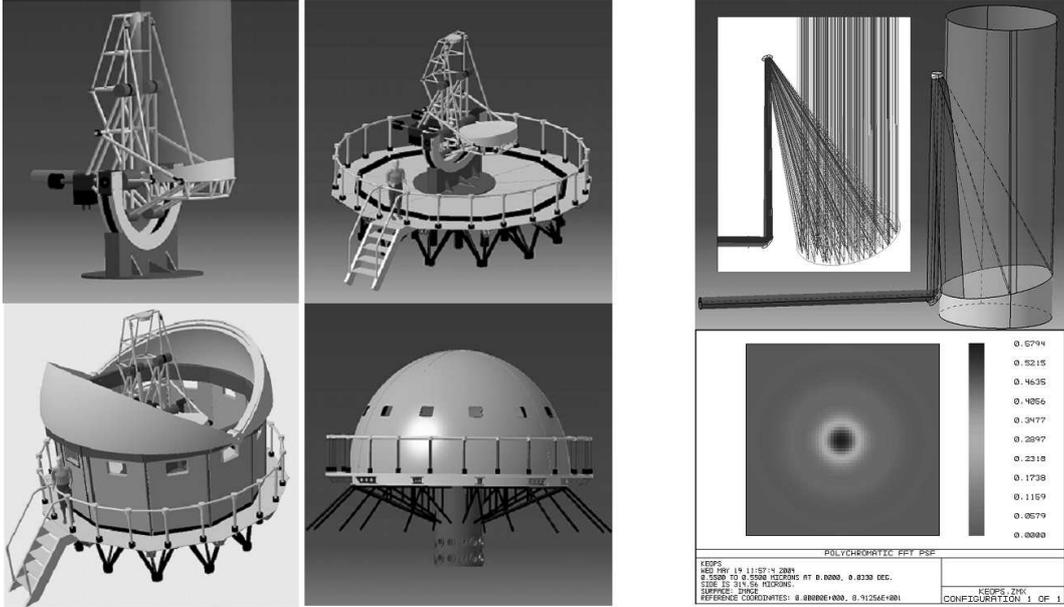
Figure 2: Different components of KEOPS: the off-axis alt-az 1.5m telescope for avoid the diffraction undesirable patterns of a classical on-axis telescope and minimizing thermal emission, its plate-form and dome, the central beam-combiner and the ray tracing for a 20" transported afocal beam within this beam-combiner.
