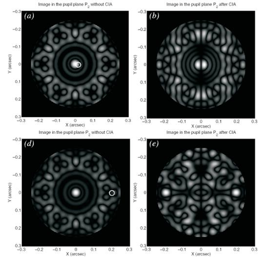
Figure 4: The snapshot imaging capability of KEOPS could be used with an Achromatic Interferential Coronagraph (Gay & Rabbia, 1996, on the left). The inversion of the pupil conduct to the total extinction of the star on the optical axis, and the apparition of the faint companion, either very close of the central star (top right) or far from the star (bottom right).
