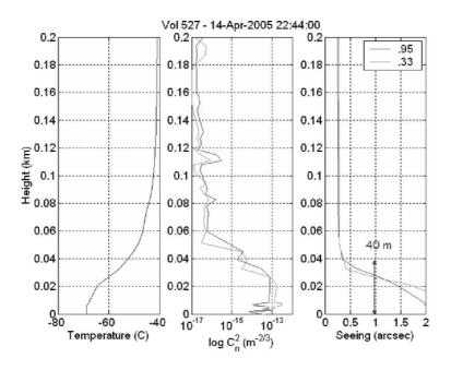
Figure 2: Example of balloons measurement; the right curve is the Temperature as function of altitude, the middle curve is the refractive index structure constant  $C_n^2$  and the left curve is the seeing (integrated from the  $C_n^2$ ). These graphics show a boundery layer limited to 40 m.
