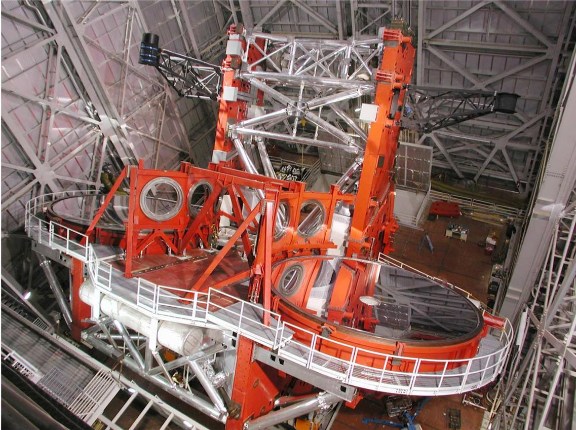
Figure 3: The Large Binocular Telescope in early 2006. This view shows the first-light prime focus camera above the left-hand primary mirror. The beam combining instruments, including LINC-NIRVANA, will occupy the central instrument platform between the two mirror cells.
