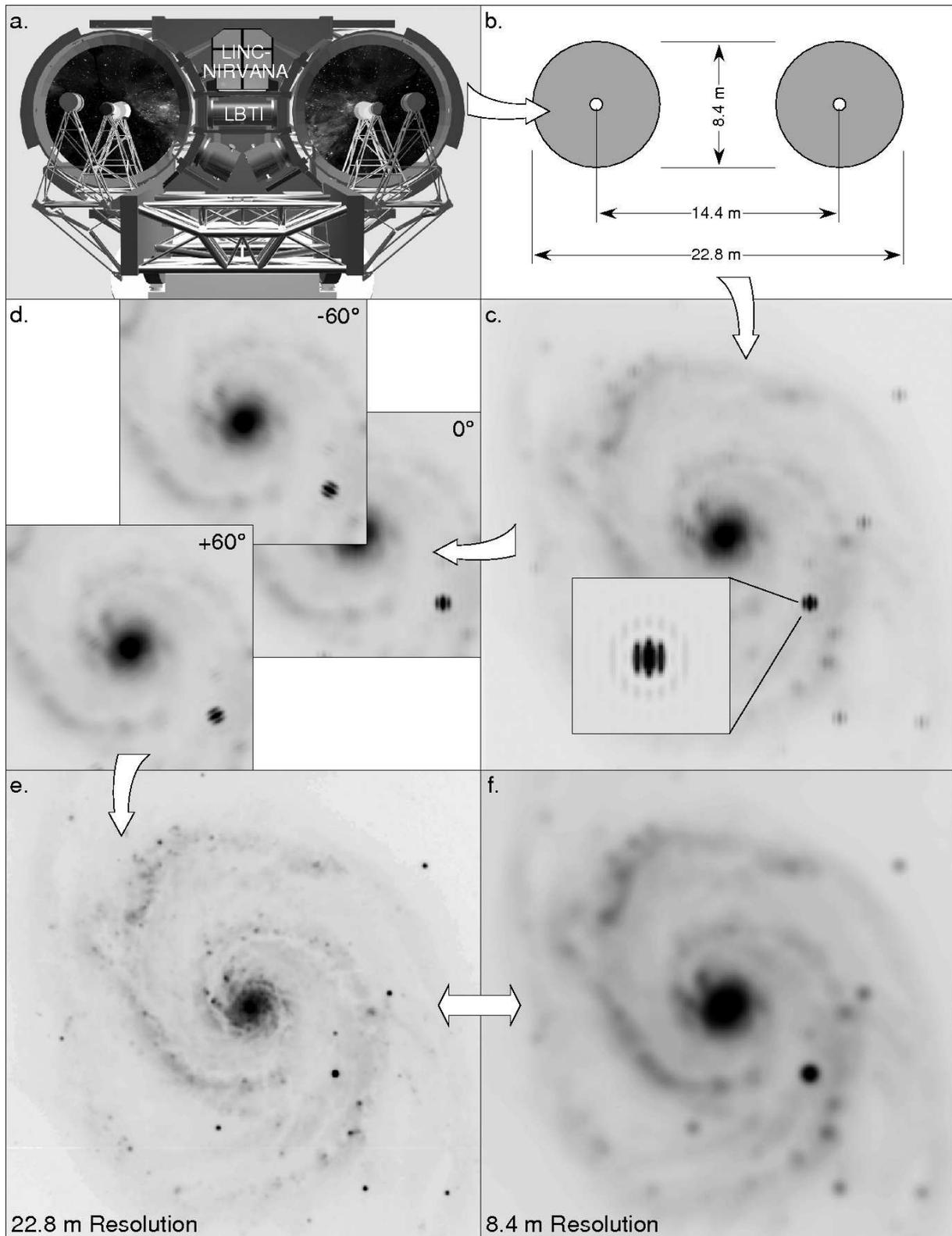
Figure 4: The principle of Fizeau imagery with LINC-NIRVANA on LBT. The entrance pupil of the telescope (panels a, b) creates a hybrid point spread function consisting of an 8.4 meter airy disk crossed by high angular resolution fringes (c). By taking several exposures at different parallactic angles (d), the observer can reconstruct the full 22.8 meter spatial resolution image. A comparison of panels e and f dramatizes the improvement over single-telescope operation.
