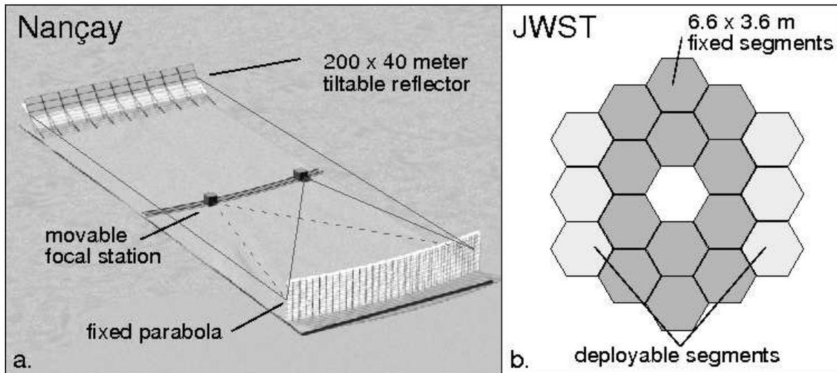
Figure 6: Other unconventional pupils in astronomy. The Nançay radio telescope (panel a) consists of a tiltable, flat reflector, a fixed parabolic primary, and a movable focal station. The primary mirror of the James Webb Space Telescope (panel b) is  $6.6 \times 3.6$  m at launch. Deployment failure of the two additional sets of 3 segments would still allow observations with the full, 6.6 m, spatial resolution of the telescope.
