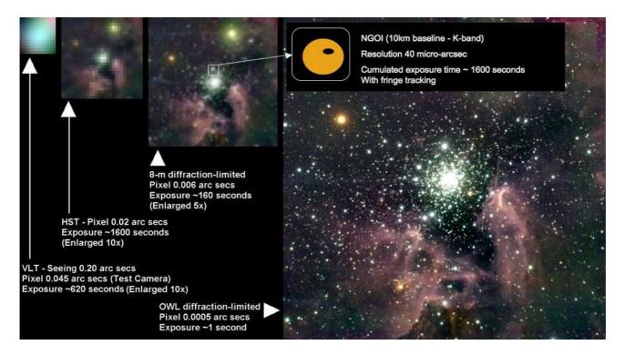
Figure 1: Resolution and sensitivity of different type of telescope: 8-meter-class ground-based seeing-limited telescope, 2-meter-class space telescope, 8-meter-class diffraction limited telescope and 100-meter-class diffraction limited telescope (courtesy ESO OWL team). The resolution and field of view of an NGOI is superimposed as a resolved elongated star with a spot.
