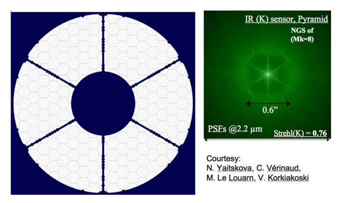
Figure 2: Typical simulated PSF (right) of an adaptive corrected OWL segmented pupil (left). The main PSF structure arise from the so-called *missing segments* (segments behind the mechanical support structure of the secondary mirror, in six-fold symmetry), from the secondary and primary mirror segmentation. The PSF is displayed in logarithmic scale.
