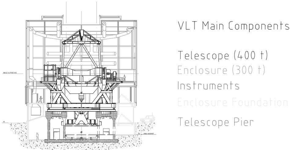
Figure 5: Cross section of VLT with main components
