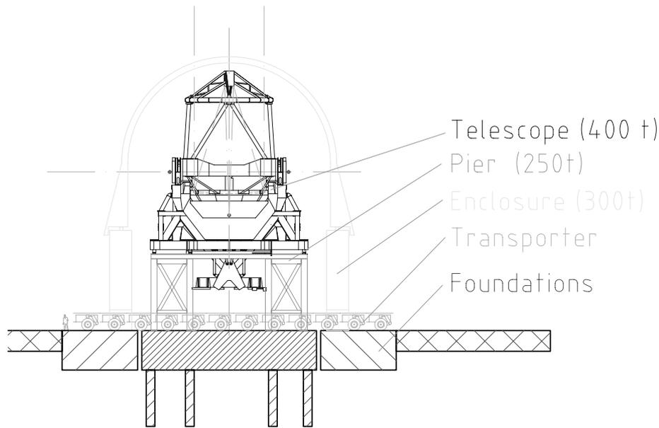
Figure 6: Strawman design of a transportable VLT
