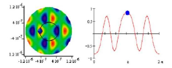
Figure 4: Transmission pattern (instanteaneous and with rotation) of a TTN array demonstrating the transmission pattern of the interferometer on the sky. Rotation modulates the signal and allow the interpretation of complex morphologies
