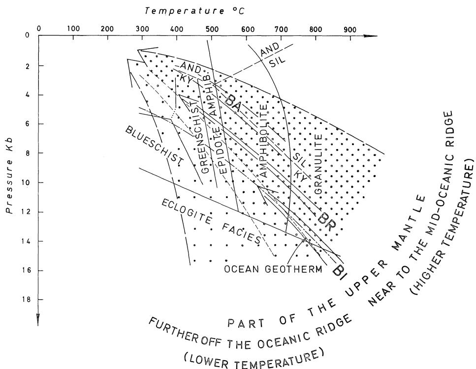
Fig. 2. — Metamorphic series in metamorphics originated by contact dynamo-thermal metamorphism related to ultramafics. The diagram of metamorphic facies is from Hyndman (1972, fig. 8-2), simplified and extrapolated to 1100° and 16 Kb. The stability limits of sillimanite (SI), andalusite (AN) and kyanite (KY) after Hyndman (1972, fig. 7-11). The oceanic geotherm after Ringwood (1969, fig. 2). BA — Banija, BR — Brezovica, BI — Bistrica.
